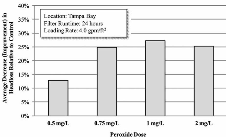
Figure 4. Average Hydraulic Performance of GAC Biofilters Supplemented With Varying Doses of Hydrogen Peroxide Relative to the Control Biofilter (No Peroxide)
