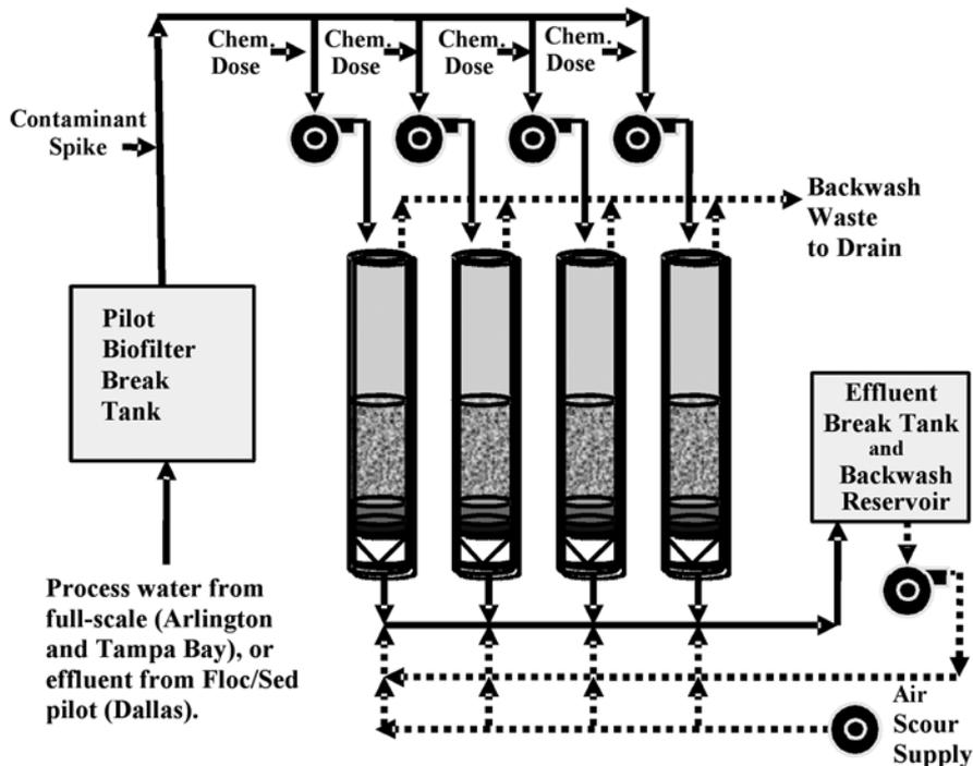
Figure 1. Biofilter Pilot Process Flow Schematic
