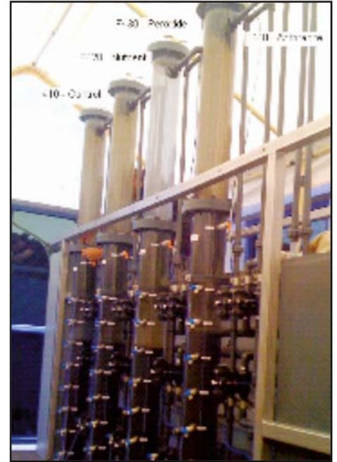
Figure 5. Photo Showing Inhibition of Algae Growth in the Biofilter Supplemented With Hydrogen Peroxide (Third Column From the Left)
